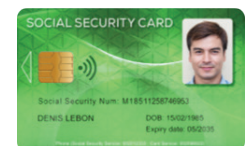
Card printed with new YMCKOO ribbon after 300 abrasion cycles (Taber test)
