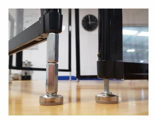
3. Once the screen is in position, adjust the feet so the screen is level and stable.
