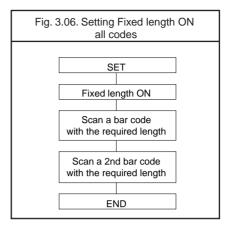
It is possible to configure a fixed length or a minimum and a maximum length for selected symbologies by reading the respective option followed by a barcode label with the required length. The different functions may be combined and will be used as follows:
